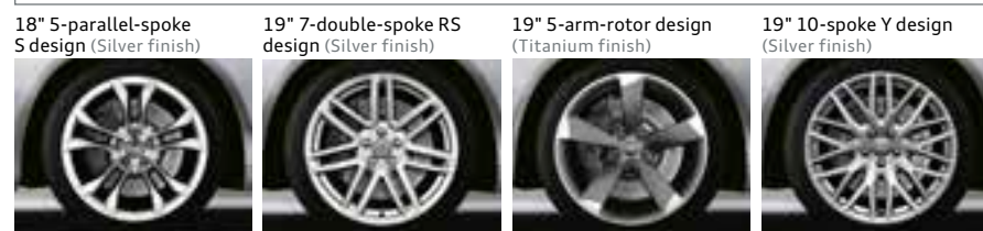
18" 5-parallel-spoke S design (Silver finish) 245/40 summer performance tires 1 or available all-season tires (Coupe) 19" 7-double-spoke RS design (Silver finish) 255/35 summer performance tires 1 19" 5-arm-rotor design (Titanium finish) 255/35 summer performance tires 1 19" 10-spoke Y design (Silver finish) 255/35 summer performance tires 1
