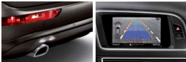
Parking system plus with front and rear acoustic parking sensors Parking system plus with rear view camera parking sensors
