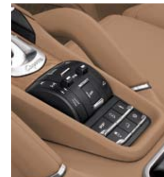
Main off-road control
