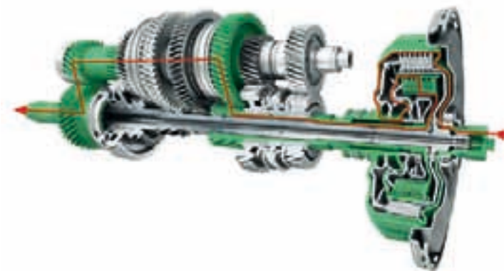
Power flow in 2nd gear
