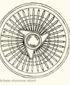
WHEELS AND TIRES: New wheel covers highlight the 1965 Sting Ray, simulating cast magnesium racing wheels with knock-off hubs. Cast aluminum wheels can be specified with wide-base six-inch rims, pin drive, and genuine knock-off type hubs. Standard wheels are 15 x 5.5K welded steel slotted disc type with 7.75 x 15 tires.
